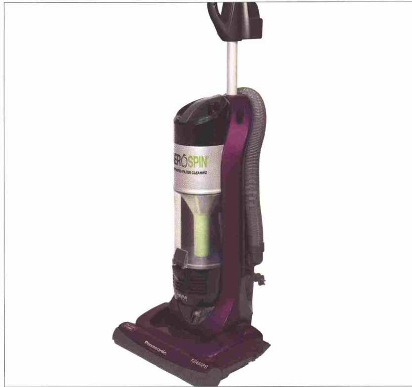
Panasonic's AeroSpin bagless upright platform uses cord retraction in a new way. Pulling the cord from the automatic cord rewind system spins the upright's filter, shaking free dust and dirt.
